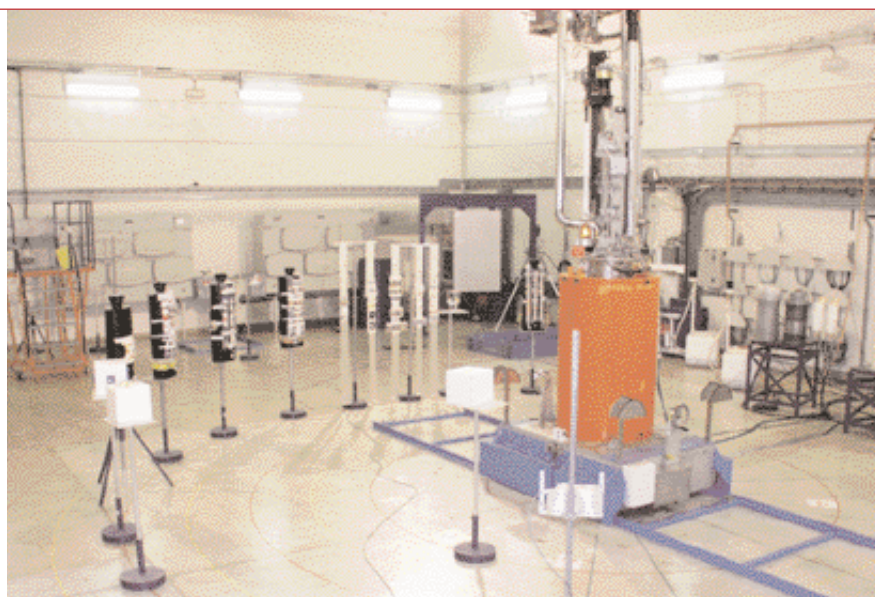
Criticality dosimeters exposed around the Silène reactor.
