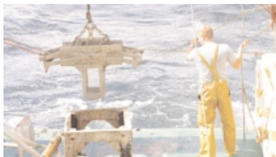
DIAPLU mission: the Flucha core sampler takes samplings for analyzing sediment.
