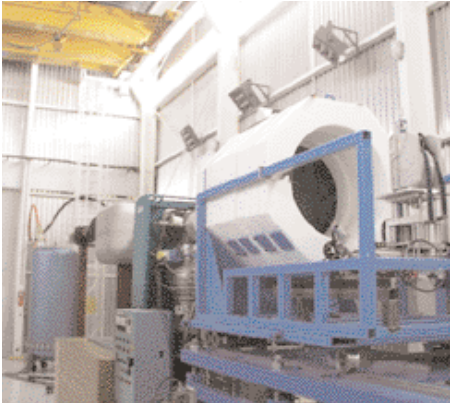
IRSN has unique tools in France for neutron dosimetry such as the CANEL moderator device shown here.
