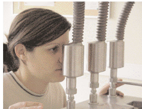
Panelist sniffing the olfactometer sniffing ports.
