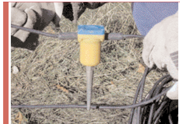
Geophone used for seismic recording.
