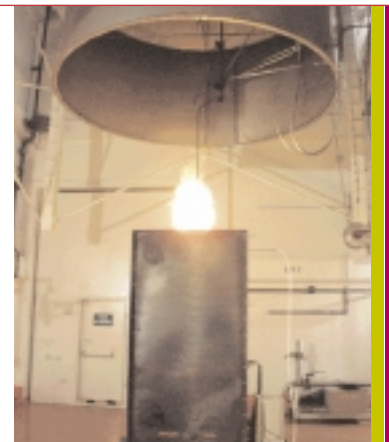
Test of the CARMELA programme for studying the combustion of electric cabinets.
