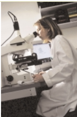
Scoring of chromosome aberrations with microscope.
