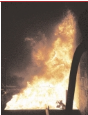
Solvent pool fire test of the FLIP (Liquid fuel fire interacting with a wall) programme.
