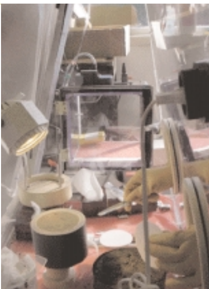
Extraction of interstitial water of sediments sampled in sea.
