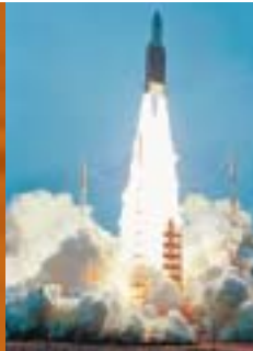
A programming error in an electrical component caused the explosion of the Ariane 501 launcher, shown here during launch from the Guyana Space Centre.
