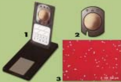
(1) Example of dosimeter fitted for radon detection, consisting of a film (2) being sensitive to particles emitted by radon, which print traces, the automatic count of these traces (3) on the film provides the measurement.
