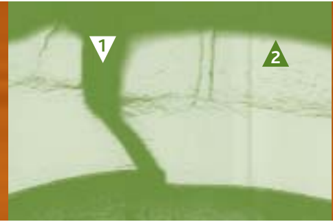
1 – Crack in clad. 2 – Hydride concentration in the Zircaloy-4 fuel rod clad used for test REP Na 8.
