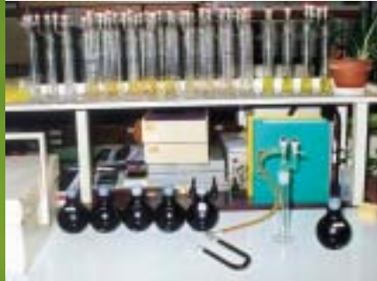
Device for radium 226 measurement via emanation, used for radiological control of drinkable waters.
