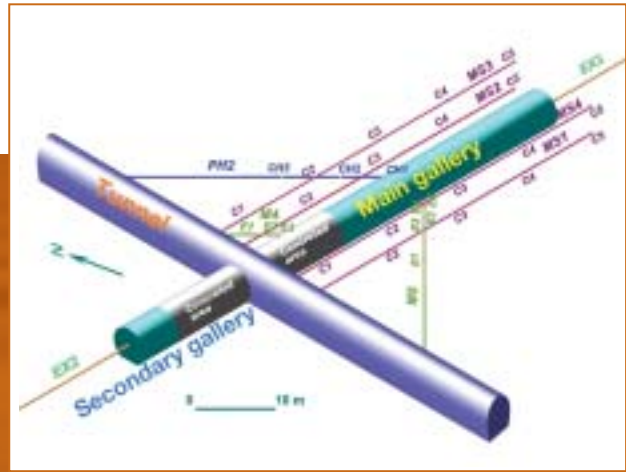
Layout of galleries and instrumentation in bores to analyse the impact of excavation of the Tournemire tunnel (Aveyron) in the argillaceous medium.
