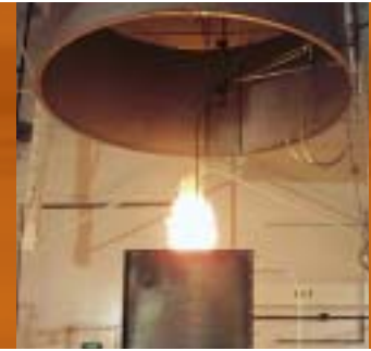
Test of the CARMELA program for studying the combustion of electric cabinets.
