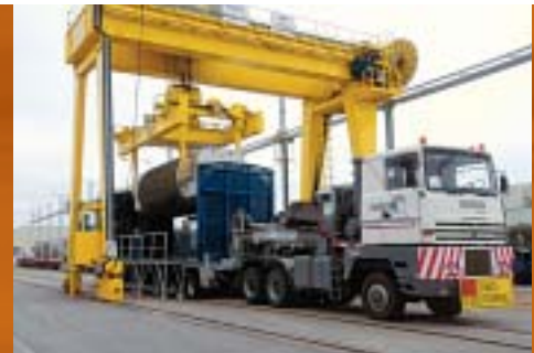
Transportation of spent fuel packages at the Valognes (Manche) railway terminal.
