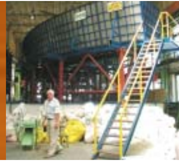
MANON loop: Study of horizontal transfer and settling at the bottom of the reactor building.
