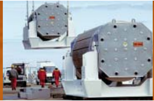
Loading a ship transporting MOX fuel packages, between Japan, La Hague and Cherbourg (Manche).
