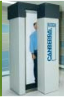
Whole-body gamma measurement: detection of external and/or internal radionuclides in the Blayais (Gironde) plant.
