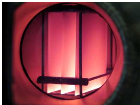
Figure 1 Catalyst sheets recombining hydrogen.
