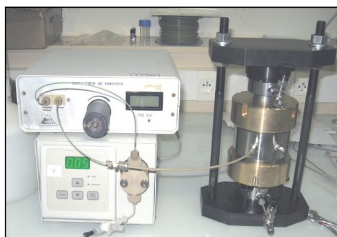
Figure 1 : cellule de percolation
