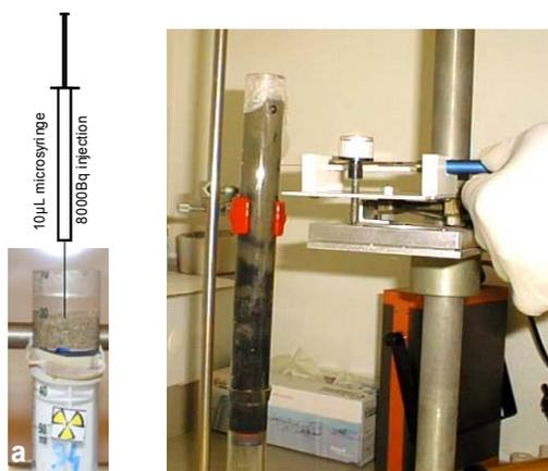
**Figure 2.** Plutonium spiking of surficial sediments (a) and of undisturbed sub-cores (b).
